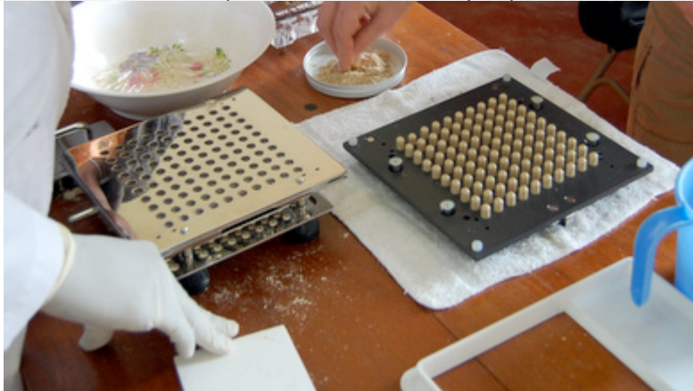
The machine helps to ensure that every capsule has the same amount of herb powder.
