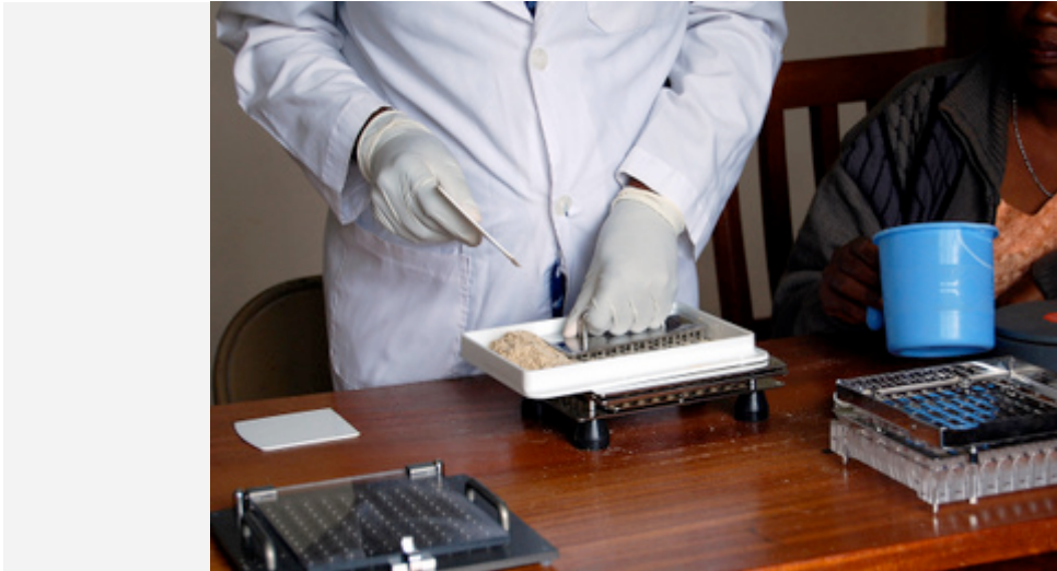
The machine helps to ensure that every capsule has the same amount of herb powder.
